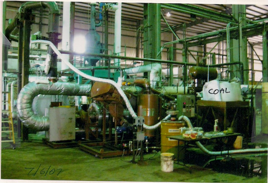
Nucor Steel Company's Carbonite Pilot Plant designed and operated by Dr. Wolfe in Conway, Arkansas in 2007-2008 at 300 pounds of coal per hour to prove out the process.
