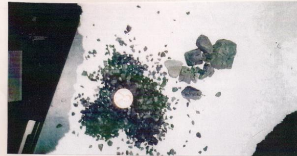
Figure 7. Fracturing of the larger top sized PRB coals along with the one-quarter inch top size coal product.
