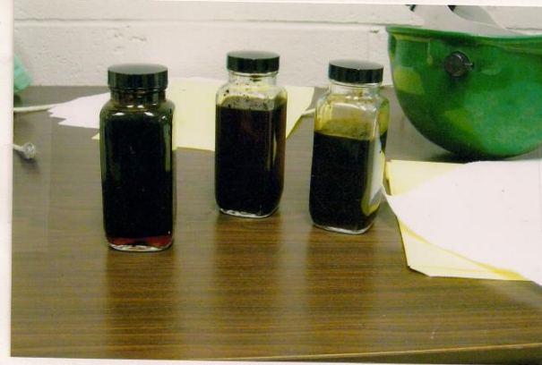
Photos of the Coal Liquids collected from the first and second condenser
